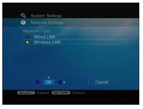
By means of the directional buttons on the remote control, select the wireless LAN option and confirm with the SELECT button.
