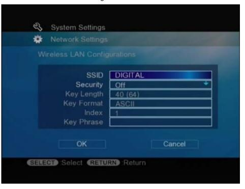
The system will go back to the main **Wireless LAN configuration page** and, at this point you will note that the name which has been assigned to SSID is registered.
