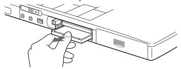
When you use a Type III PC card, you need to remove both the top and bottom PC card slot protectors
