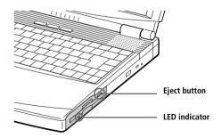
If you have difficulty removing a diskette from the floppy disk drive, remove the floppy disk drive from the multi-purpose bay.
