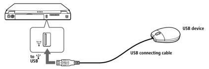
△ USB ports are included to provide state-of-the-art technology. You may need to install software (device drivers) supplied with your USB device before using the USB device.
