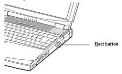
Place a DVD- / CD-ROM disc in the tray with the label side facing up. For DVD discs, which can be played on both sides, the side of the disc facing up is the side that plays. Push the disc onto the hub until the disc clicks into place.
