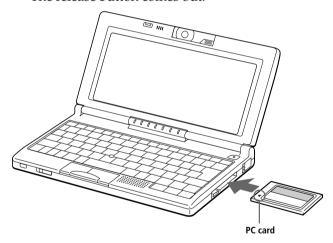
Do not force a card into the slot. It may damage the connector pins.
