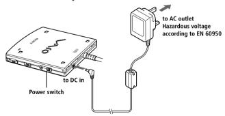
AC adapter cable (SELV, according to EN 60950)
