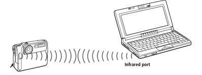
When performing a data transfer with any software using infrared, enable the IrDA in the Control panel of Windows, as follows (Do not use the icon in the taskbar):
