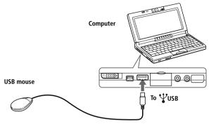
USB ports are included to provide state-of-the-art technology. You may need to install software (device drivers) supplied with your USB device before using the USB device. See the manual that came with your mouse for more information on installation and use.
