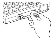
Insert the PC card into the PC card slot, front label facing up. Gently push the card into the slot until the card is fixed into the connector.
