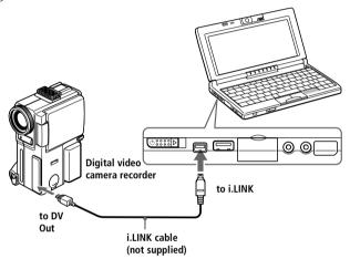
The Sony digital video camera recorder (DCR-PC1) is pictured; your digital video camera recorder may need to be connected differently.
