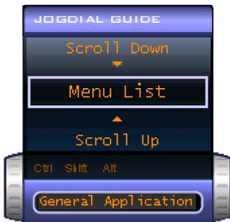
The Center Jog Control window switches to Guide mode when you start an application and its window becomes active. Depending on the application, the Center Jog Control window displays different commands that you can select or execute by rotating or pressing the Center Jog Control.
