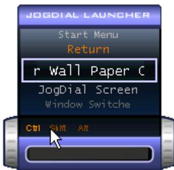
The Center Jog Control window is in Launcher mode until you start an application or the Center Jog Control window becomes active. When an arrow appears next to an item in the Center Jog Control window, you can display a submenu for that item by selecting it and pressing the Center Jog Control.
