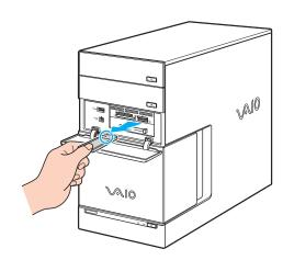
You are recommended to remove the memory stick before shutting down the computer.
