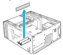
7 To insert a new memory module, remove it from its anti-static package, handling it only by the edges.
