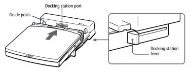
5 Slide the docking station lever into the LOCK position to secure your computer in the docking station.
