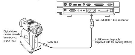
Sony's digital video camera recorder (DCR-PC7) is pictured; your digital video camera recorder may need to be connected differently.
