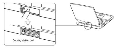
3 Align the indentation on the bottom of the computer with the guide post on the docking station.
