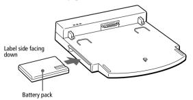
When the battery pack is fully inserted, close the cover.
