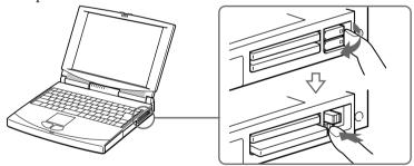
Remove the PC card slot protector. When you use a Type III PC card, you need to remove both the top and bottom PC card slot protectors.
