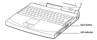
If you have difficulty removing a diskette from the floppy disk drive, remove the floppy disk drive from the multi-purpose bay.
