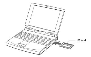
Do not force a card into the slot. It may damage the connector pins.
