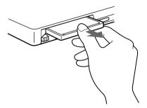
Insert the PC card into the PC card slot, front label facing up. Gently push the card into the slot until the card is fixed into the connector. The release button comes out.
