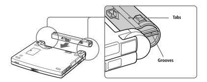
Slide the lock lever into the LOCK position to secure the battery on the computer.
