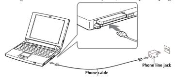
Use the supplied communication tools which provide a full range of features: fax, data... See "About Your Sony Notebook Computer" for details. Phone cable and connectors: TNV (Telecommunication Network Voltage), according to EN60950.
