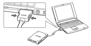
Fold the floppy disk drive cable into the compartment on the side of the floppy disk drive.
