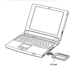
Do not force a card into the slot. It may damage the connector pins.
