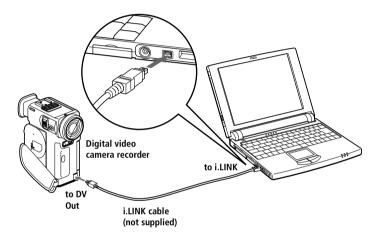
The Sony digital video camera recorder (DCR-PC7) is pictured; your digital video camera recorder may need to be connected differently.
