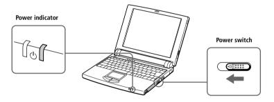
All fyou hold the power switch in the on position for more than four seconds, the computer turns off.
