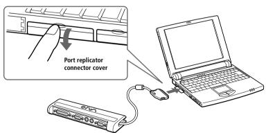
Plug the port replicator cable into the port replicator connector on the computer.
