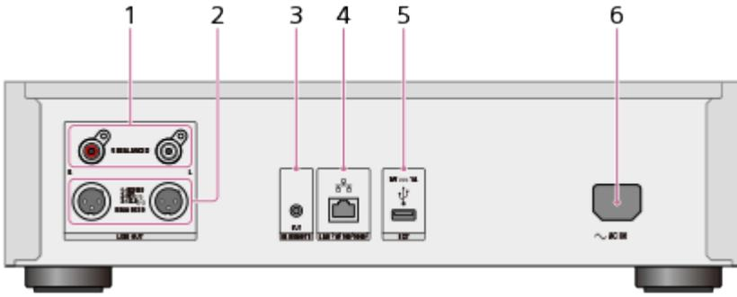
1. LINE OUT UNBALANCED (analog: unbalanced output) L/R jacks
