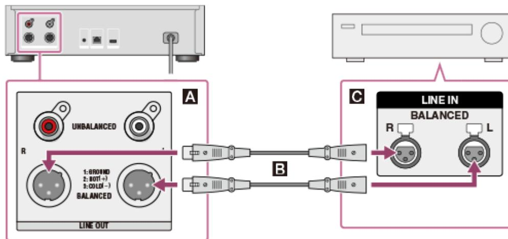
**A**: LINE OUT UNBALANCED L/R jacks of the HDD AUDIO PLAYER
