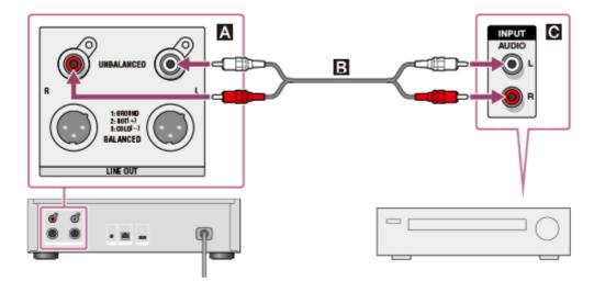
A: LINE OUT UNBALANCED L/R jacks of the HDD AUDIO PLAYER
