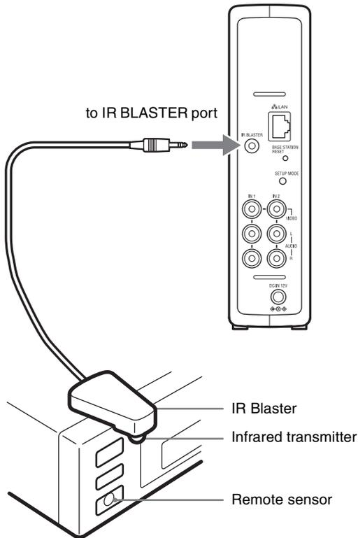
With reference to the operating instructions of the device, make sure to place the IR Blaster just above the remote sensor.
