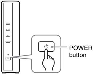
The POWER LED on the front panel of the Base Station lights green.
