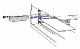
6 Install the add-on board by plugging it into the expansion slot and secure it with the screw from the expansion slot, as shown:
