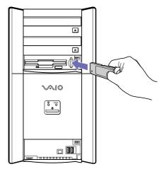
Always hold the Memory Stick™ with the arrow pointing in the correct direction when you insert it into the slot. To avoid damaging the computer or the Memory Stick™, do not force the Memory Stick™ into the slot if it does not insert smoothly.
