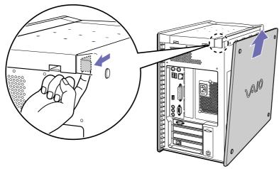
Always wait for the internal parts of the system unit to cool down before removing the side panel.
