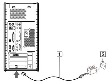
A country-specific phone plug is supplied with your VAIO desktop, allowing you to plug the phone line into the wall jack. We recommend you to use the supplied plug, because the usage of any other phone plug can decrease the connection quality.
