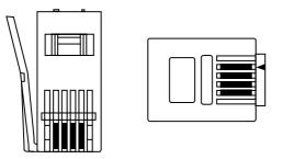
Use the plug already attached to the phone cable. The connector can be identified by its cuboid shape and flat pins:
