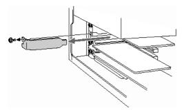
6 Install the add-on board by plugging it into the expansion slot and secure it with the screw from the expansion slot, as shown (configuration may vary):
