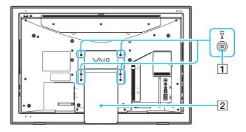
**3** Use the four holes (3) for mounting by following the instructions described in the manual that came with your mounting system.
