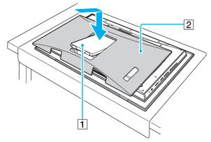
2 Align the cover with the back of the computer and push it in.
