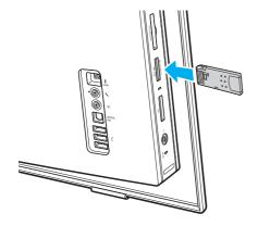
Be sure to hold the Memory Stick media with the arrow pointing in the correct direction as you insert it into the slot. To avoid damaging your computer or the Memory Stick media, do not force the Memory Stick media into the slot if you cannot insert it smoothly.
