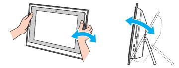
While adjusting the viewing angle, do not exert excessive pressure on your computer, especially on the center of the speaker grill, to eliminate a risk of mechanical damage.
