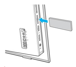
Insert the ExpressCard slot protector to protect against debris entering the slot when not using an ExpressCard module. Before moving your computer, be sure to insert the ExpressCard slot protector into the slot.
