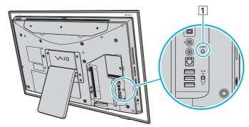
6 Press the **CONNECT** button on the bottom of the mouse within 10 seconds from step 5. Communication between the mouse and the computer should now be established.
