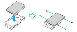
A new hard disk drive comes with the necessary screws. Do not overtighten these screws when securing the drive to the drive holder.
