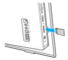
3 Carefully slide the memory card into the slot until it clicks into place. Do not force the card into the slot.
