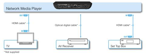
– When this player and the TV are connected with HDMI cables via an AV Receiver, pictures may not be displayed properly due to the copyright protection feature of some Set Top Boxes. In this case, contact your Cable/Satellite TV Operators.
