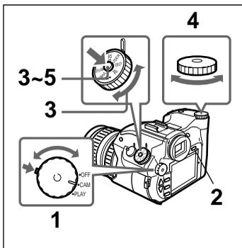
**1** While pressing the mode lock (green), turn the power/mode dial to CAM mode.
