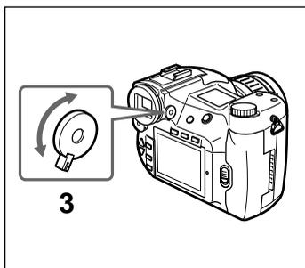
**3** Turn the eyesight adjustment lever to where you can clearly see the circle in the center of the viewfinder.
