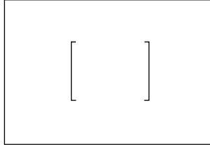
Selecting the “Guide 90” frame changes frame display to guide lines that can be moved horizontally. These guide lines can be used to establish horizontal subject size and positioning within the frame.
