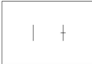
Selecting the “Guide 0” frame changes frame display to guide lines that can be moved vertically. These guide lines can be used to establish vertical subject size and positioning within the frame.
