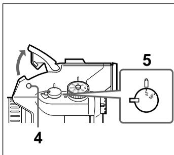
**4** If there is insufficient light to shoot the subject (shutter speed or F-stop flashes), press the flash pop-up key to open the flash.
