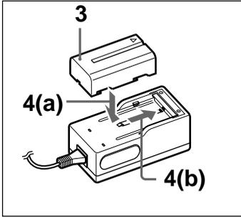
**3** Making sure the ▲ mark is pointed in the right direction, place the battery pack in the hollow of the battery charger.
