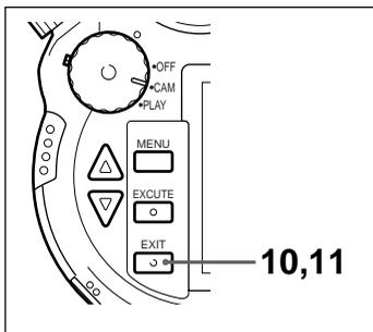
**9** If you finish inputting the keyword before reaching the 16-letter limit, move the cursor to END and press the EXECUTE button.
