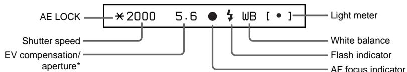
\* The EV compensation is displayed when EV Button is pressed.
