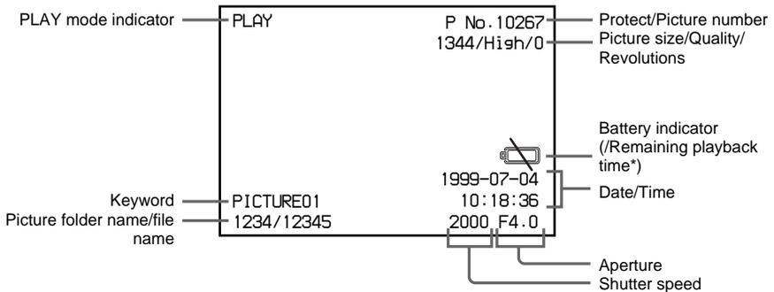
\* Usually remaining playback time is displayed. When the battery gets weak, the battery indicator flashes. The remaining playback time is not displayed when using AC power adaptor/charger AC-V700.
