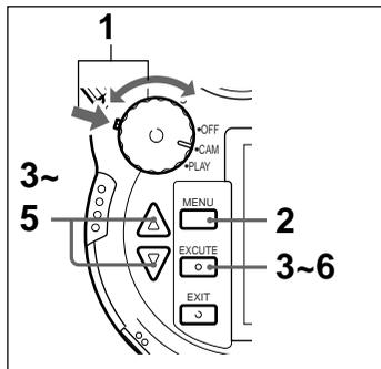
**1** While pressing the mode lock (green), turn the power/mode dial to CAM mode.
