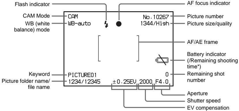
\* Remaining shooting time is not displayed when using AC power adaptor/charger AC-V700. Usually the remaining shooting time is displayed. When the battery gets weak, the battery indicator flashes.
