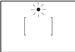
When the picture is focused, the indicator lights a steady green. If the picture cannot be focused, the indicator lights a steady red.
