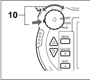
**10** Turning the power/mode dial to OFF turns the power off.
