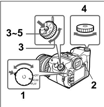
**1** While pressing the mode lock (green), turn the power/mode dial to CAM mode.
