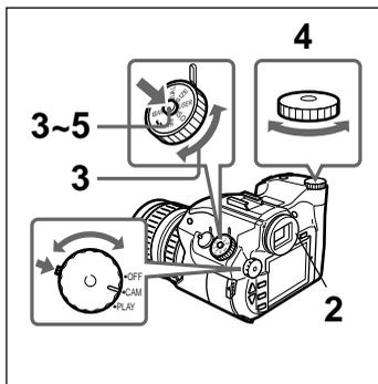
**1** While pressing the mode lock (green), turn the power/mode dial to CAM.
