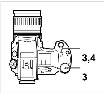
**1** While pressing the mode lock (green), turn the power/mode dial to CAM.
