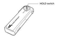
Tune the HOLD switch in the direction of the arrow.
