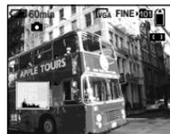
**Adjusting the exposure to the + side shifts the histogram to the right side.**
