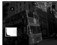
**Adjusting the exposure to the – side shifts the histogram to the left side.**
