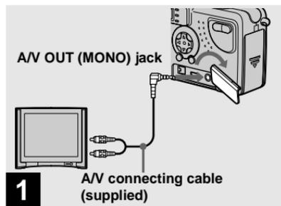
→ Using the A/V connecting cable, connect the A/V OUT (MONO) jack of the camera to the audio/video input jacks of the TV set.
