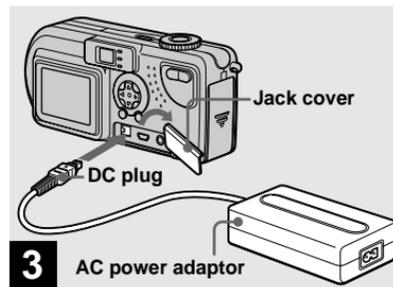
➔ **Open the jack cover, and connect the AC-LS1A AC power adaptor (supplied) to the DC IN jack of the camera.**
