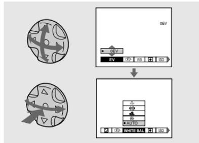
To change the current settings of the camera, bring up the menu or the SET UP screen (page 50), and use the control button to make the changes.
