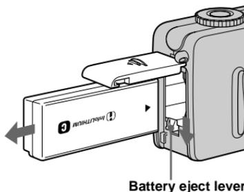
Open the battery/"Memory Stick" cover, and push down the battery eject lever in the arrow direction as illustrated above.
