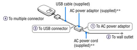
**NW-A1000**: The battery charges to about 80% in approximately 1 hour\*, a full charge requires approximately 2 hours.\*
