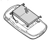
6 Pull the cord connecting the battery to the player to separate the battery plug from the connector.
