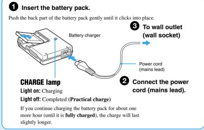
• Connect the battery charger to an easily accessible wall outlet (wall socket) close by.
