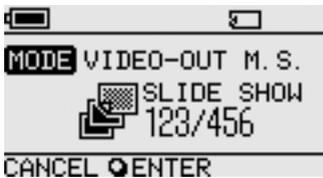
The default interval setting for slide show mode is approximately 5 seconds, but this varies according to the file size. Images are automatically switched at this rate. If desired, you can change the interval setting. For details, see “Changing the slide show time interval” on page 26.
