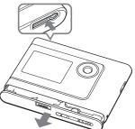
**4** Remove the screw on the side of the battery and the adhesive tape on the battery.
