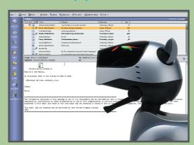
Available for ERS-210A and ERS-220A, Wireless LAN technology enables your AIBO to communicate with your PC.
