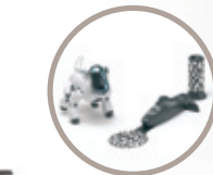
AIBO locates autonomously its energy station when its energy is dropping. The pattern on the Energy Station Pole helps AIBO to localise and position itself quickly.
