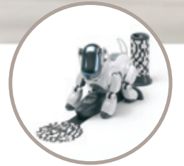
AIBO locates autonomously its energy station when its energy is dropping. The pattern on the Energy Station Pole helps AIBO to localise and position itself quickly.
