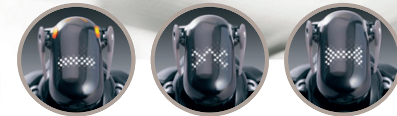
Multi-colour LEDs allow AIBO to express emotions and what it is thinking.
