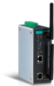
NPort W2150A 1-port RS-232/422/485 IEEE 802.11a/b/g wireless device server
