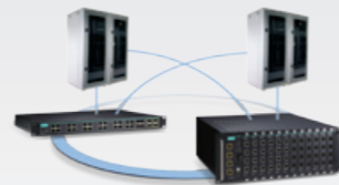
Redundant ring & uplinks
