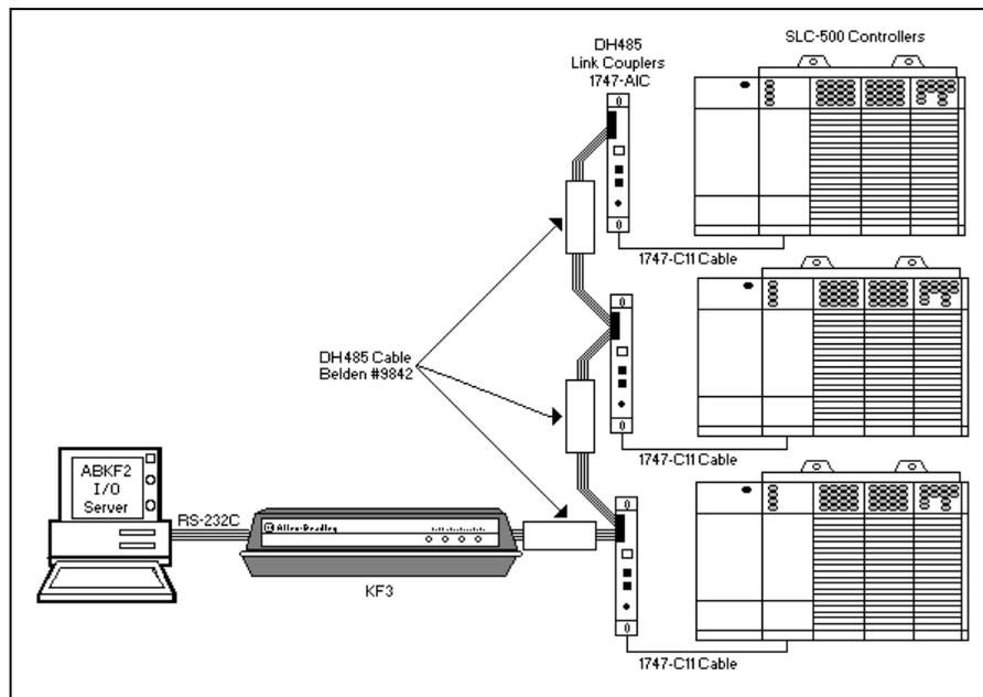
The RS-232-C cable used between the computer and the KF3 module should be pinned out as previously described.
