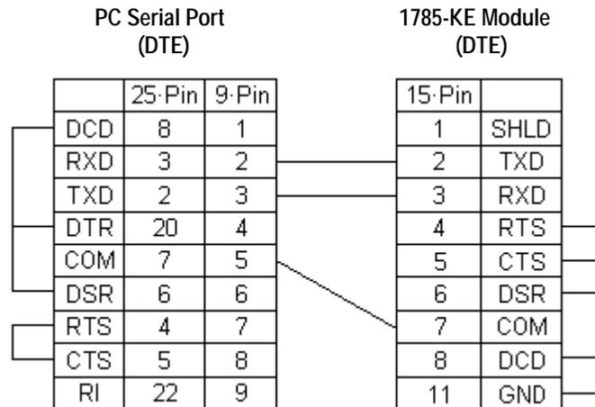
**Note** The 1785-KE module has only a 15-pin D-Shell connector. Therefore, only the 15-pin is shown.
