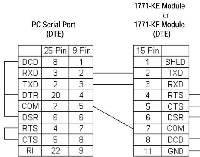
**Note** The 1771-KE and 1771-KF modules have only a 15-pin D-Shell connector. Therefore, only the 15-pin is shown.
