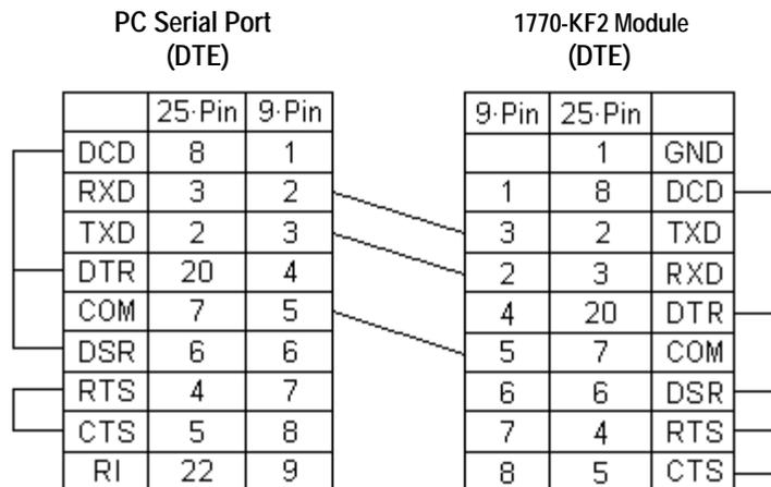
**Note** The 1770-KF2 module has only a 25-pin D-Shell connector. The 9-pin connection is shown to allow for a 9-25 converter to be used.
