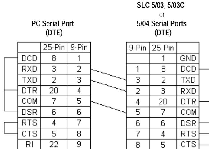
**Note** This is not the same pinout used in the Allen-Bradley 1747-CP3 cable, but a CP3 will work in this situation.
