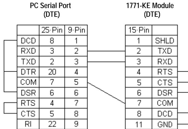
**Note** The 1771-KE module has only a 15-pin D-Shell connector. Therefore, only the 15-pin is shown.
