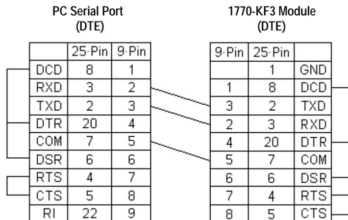
**Note** The 1770-KF3 module has only a 25-pin D-Shell connector. The 9-pin connection is shown to allow for a 9-25 converter to be used.
