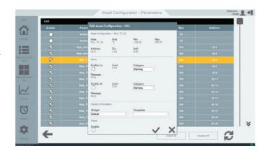
OPC: InTouch HMI - Machine Edition provides native OPC interfaces, such as OPC UA (Client/Server), OPC DA (Client/Server), OPC XML (Client), OPC .NET (Client), and OPC HDA (Server). OPC UA and OPC DA also offers native redundancy configuration.
