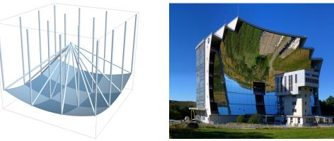
Paraboloids of this type are called "parabolic dishes" and are using to concentrate sound waves, radio waves, and light, particularly in solar energy applications, such as the solar furnace shown above right.
