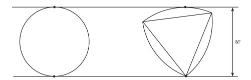
The illustration above shows two curves of constant width w (the circle and the Releaux triangle) with marked pairs of opposite points. The Releaux triangle is made up of three arcs of circles centered at the three vertices of an equilateral triangle. In each case, we see that the distance w is equal to the sum of the radii of curvature at the marked points (the bottom point on the right-hand curve is a corner point, and so has radius of curvature zero).
