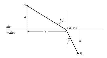
1. Write down the time T(x) required for light to complete the path shown below in terms of the variable x and the constants a, b, c, v, and s.
