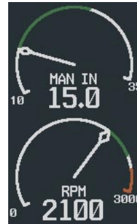
Figure 6-1 Round Dial Gauges: Manifold Pressure Gauge and Tachometer
